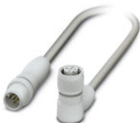
Sensor/Actuator cable, 5-position, PP-EPDM halogen-free, Gray RAL 7035, Plug straight M12, A-coded, on Socket angled M12, A-coded, Cable length: 0.6 m, Hygienic design, with plastic knurl
